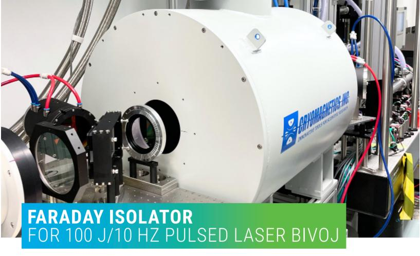
Large-aperature optical isolator based on the Faraday effect capable of reliable protection of the laser amplifier chain delivering 100 J nanosecond laser pulses at the repetition rate of 10 Hz.
