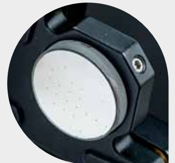
DAMAGED SURFACE OF TESTED MIRROR
