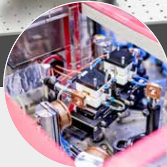
DETAIL OF THE MAIN AMPLIFIER CAVITY
