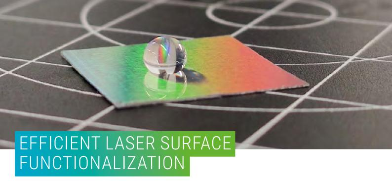
The HiLASE Centre holds two records in laser manufacturing: speed production of laser-induced periodic nanostructures on stainless steel surface reaching 1909 cm2/min, and using over 40 thousand beams in a laser multi-beam nanostructuring. These achievements make this eco-friendly technology creating new properties on the treated material surface even more attractive for industry.
