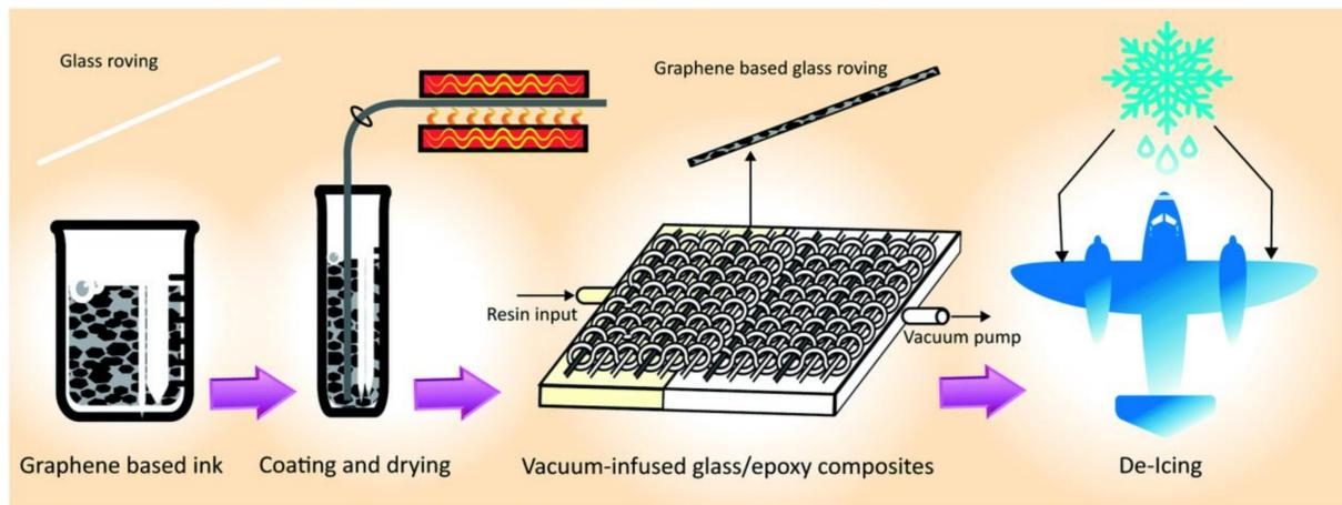
**Figure 4.** A dip-dry-cure technique for manufacturing graphene-based glass/epoxy composites for de-icing applications [63].
