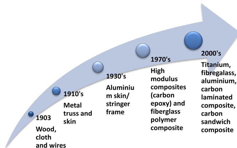
Figure 2. Evolution of materials used in the airframe structure [10–12].
