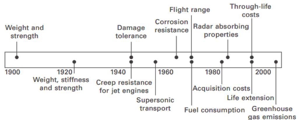
**Figure 1.** Historical timeline indicating when critical measures for materials selection were introduced into aircraft design [2].
