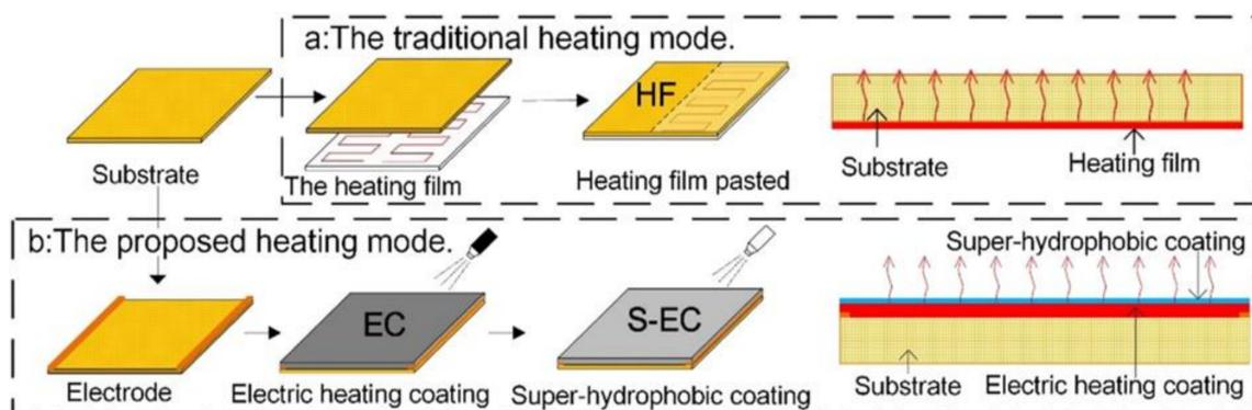
**Figure 5.** Schematic of the fabrication process and the heating mode of the samples (a) H.F. and (b) S-EC. (Reported from [64] with permission; Copyright 2018 Elsevier B.V.).
