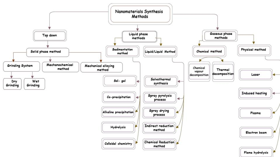
Figure 8. Different methods for generation of nanomaterials.
