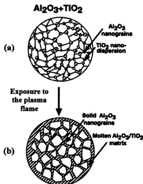
**Figure 6.** Substrates depicting (a) unexposed  $\text{Al}_2\text{O}_3\text{-TiO}_2$  nanograins and (b) morphology of  $\text{Al}_2\text{O}_3\text{-TiO}_2$  when exposed to plasma flame.
