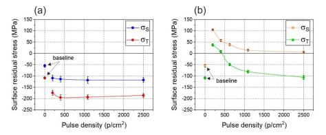
**Figure 7.** Surface residual stresses in LPwC treatments as a function of laser pulse density: (**a**) LPwC IR and (**b**) LPwC SHG.
