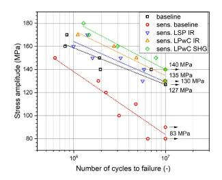
**Figure 8.** S–N curves of LSP treated sensitized AA5083 after 3-point bend test in 3.5% NaCl solution. Plots for non-sensitized samples (baseline) is provided for comparison.
