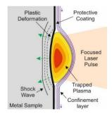
Figure 1. LSP mechanism.
