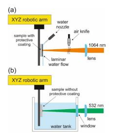
Figure 2. (a) LSP and (b) LPwC underwater setup.
