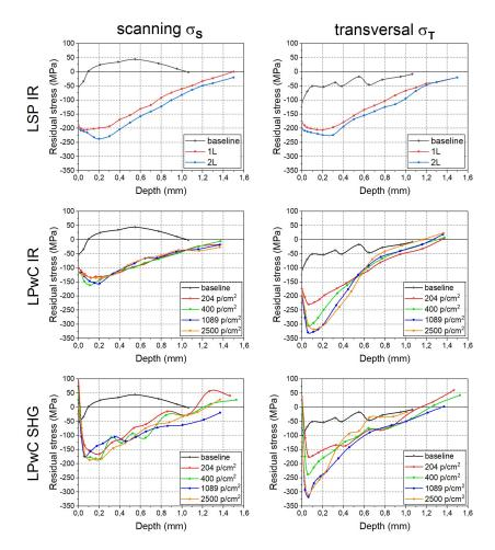
**Figure 6.** XRD residual stress measurements of selected peening setups (rows) in scanning  $\sigma_S$  and transversal  $\sigma_T$  direction (columns).
