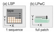
**Figure 3.** Peening strategies used: (**a**) LSP sequencing when protective coating is used and (**b**) LPwC single pass for the whole patch in the absence of coating.
