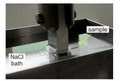
Figure 5. Corrosion fatigue 3-point bend testing setup.
