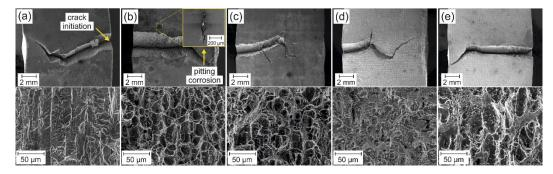
**Figure 9.** SEM images of cracked samples (**top**) and detail of the fracture surface (**bottom**) after 3-point bend testing: (**a**) baseline, (**b**) sensitized baseline, (**c**) sensitized LSP IR, (**d**) sensitized LPwC IR and (**e**) sensitized LPwC SHG.
