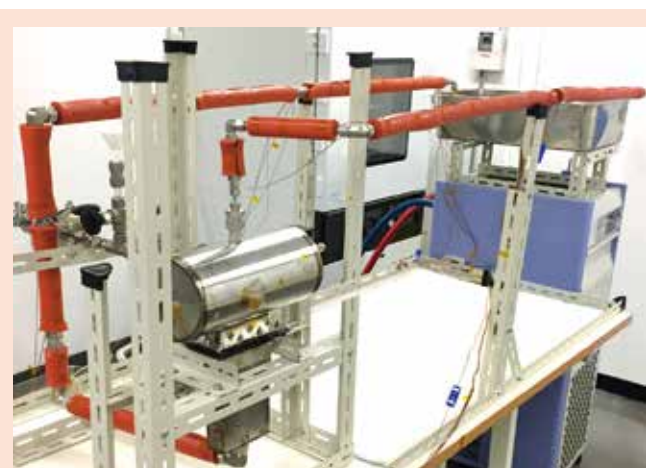
Large-capacity loop heat pipe to use untapped heat effectively
