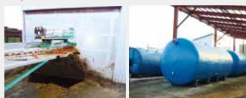
Automatic feeder and pretreatment unit for raw materials as well as an FRP methane fermentation tank (thermophilic dry fermentation)
