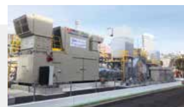
Plant for demonstrating dry low-NOx combustion with a hydrogen-fueled gas turbine
