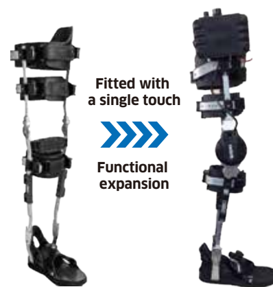
Modular Leg Brace NOE combined with Switch Knee for walking control
