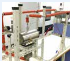
Loop heat pipe with a high heat transport capacity for harnessing untapped thermal energy
