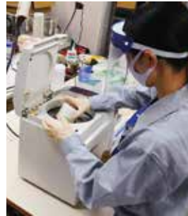
Compounding of CNFs and natural rubber using a planetary centrifugal mixer
